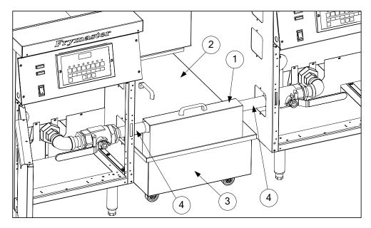
Remove the front filter pan cover and insert the oil baffle to prevent splashing and movement during filtering. The oil baffle fits straight down over the two drain tubes and rests on the hold-down ring frame.
